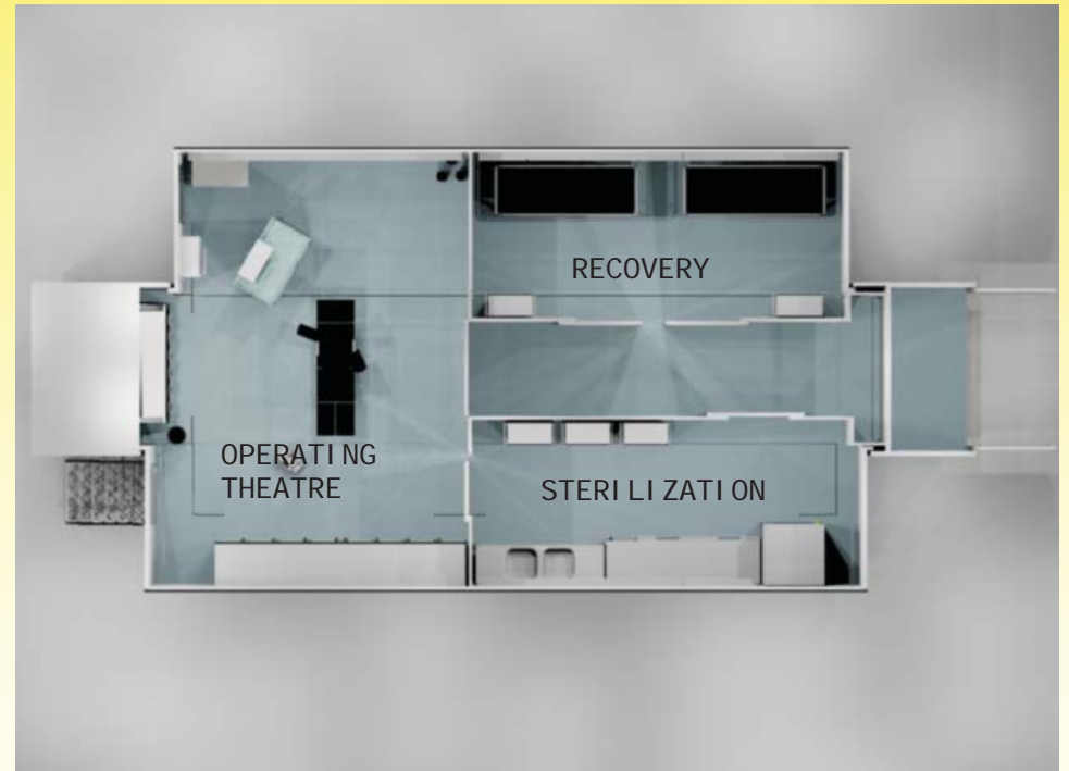
Top-view drawing of the MultiSpace unit with Operating Theatre, Recovery and sterilization.
